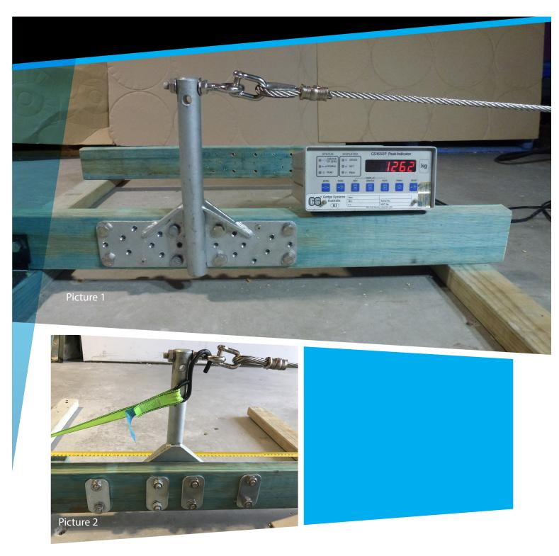
Picture 1 - Test shown above has Rafter Bracket fixed to 90 x 35mm structural pine MGP12. Load held static at 1250kgs for 7 days without failure.
